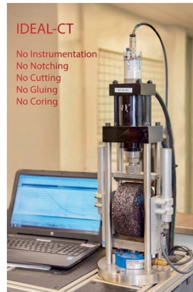
IDEAL-CT asphalt cracking test developed by Highway IDEA Project 195. The test is simple, rapid, reliable, and sensitive to asphalt mix design. It needs no instrumentation, cutting, gluing, drilling or notching of the test specimen. (Photo courtesy Inam Jawed)
