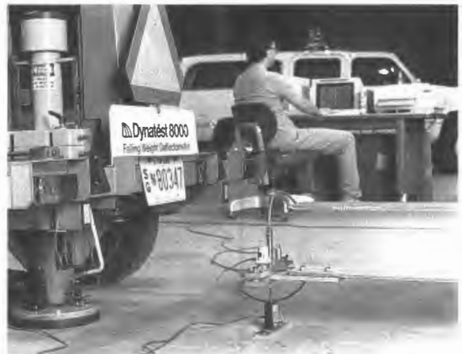
FIGURE 6 FWD deflection sensor calibration equipment.
