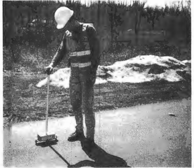
FIGURE 2 Profile data collection using the Face Technologies Dipstick.
