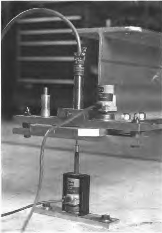
FIGURE 4 Geophone in holder (on test pad) with LVDT mounted on end of aluminum I-beam; second geophone (right of LVDT) used to monitor beam movement.
