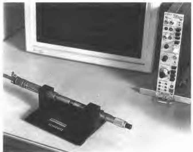
FIGURE 3 Reference LVDT in micrometer calibrator; 2310 signal conditioner to the right of computer monitor.
