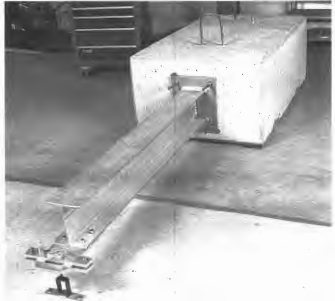
FIGURE 5 Aluminum I-beam mounted on concrete inertial block; deflection sensor holder bolted to test pad beneath end of beam. To calibrate KUAB seismometers, LVDT holder is moved to top of I-beam.
