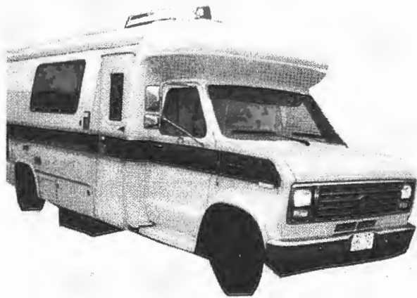
FIGURE 1 Profile data collection using the K.J. Law 690 DNC profilometer.
