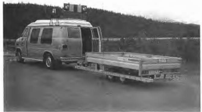
FIGURE 1 Equipment for measuring rut depth, crossfall, and road roughness.
