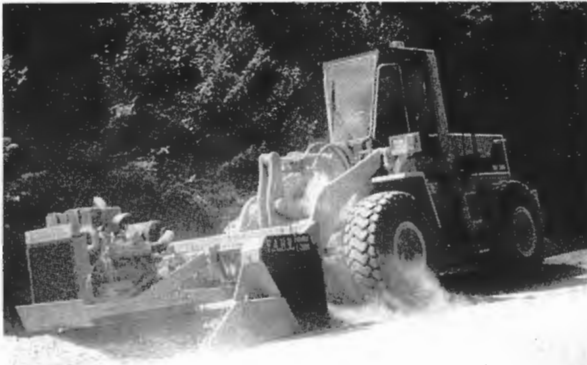
FIGURE 3 F.A.H.R. single-rotor crusher retrofitted to a front-end loader.
