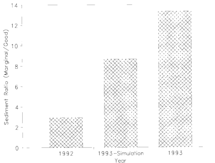
FIGURE 3 Ratio of marginal-quality aggregate sediment production to good-quality aggregate sediment production for 1992 natural rainfall, 1993 rainfall simulation, and 1993 natural rainfall. Simulation represents a 50-mm/hr storm for 30 min.
