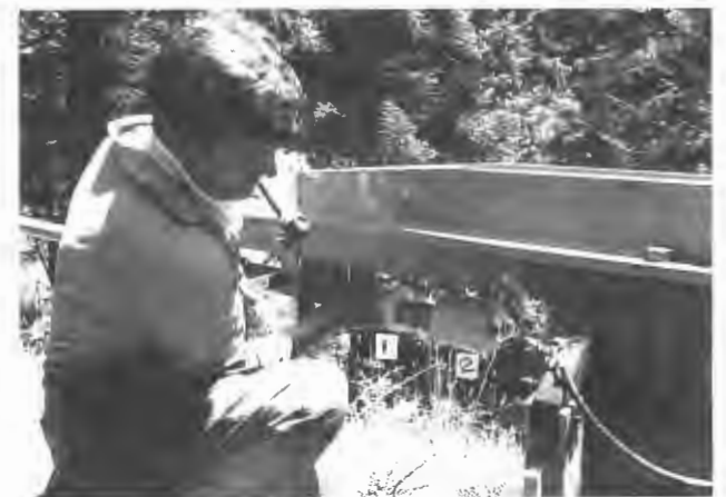
FIGURE 6 Soil nail ready for insertion loading into launcher. Compressed air is introduced between locking washer (1) and collet (2). The collet separates from nail in noise and debris shroud.
