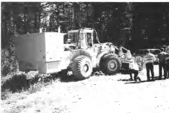
FIGURE 1 Roto Trimmer mounted on a Caterpillar loader (rotary drum on front lift arms and power pack at rear).
