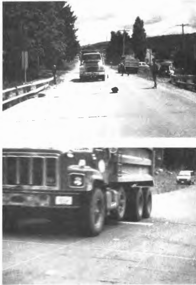
FIGURE 6 Artificial bump at bridge entrance.
