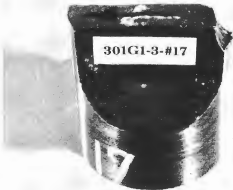
FIGURE 7 Core 17 showing transverse weld metal crack extending into flange; Cores 23 and 25 are similar. Arrow on web indicates west direction.
