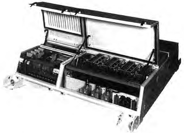
FIGURE 6 Compact and lightweight, roof-mounted AC traction inverter unit.
