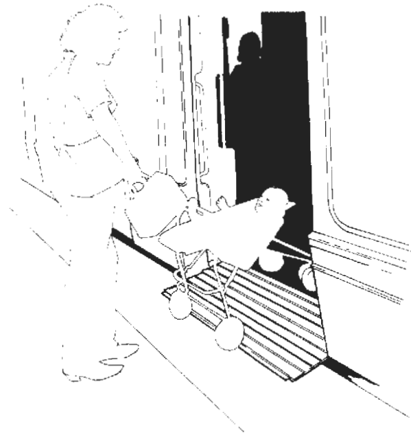
FIGURE 8 Powered ramp on GEC Alstom low-floor LRVs in Nantes, France. Ramp is deployed within a fraction of a second, together with opening door.
