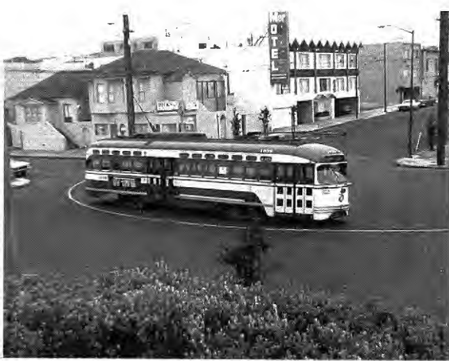
FIGURE 5 The PCC streetcar was developed by a committee of presidents of transit operating companies. Standardized cars of this type were manufactured by two builders between 1937 and 1952.
