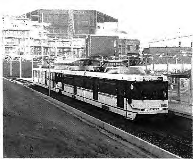
FIGURE 6 The high-floor articulated Model U-2 car by Siemens-Duewag operates on several North American light rail lines, including St. Louis.
