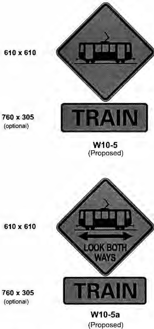
FIGURE 2 LRT crossing signs [colors: symbol, arrow, legend, and border—black (nonreflecting); background—yellow (reflective); dimensions in millimeters; 25.4 mm = 1 in.].
