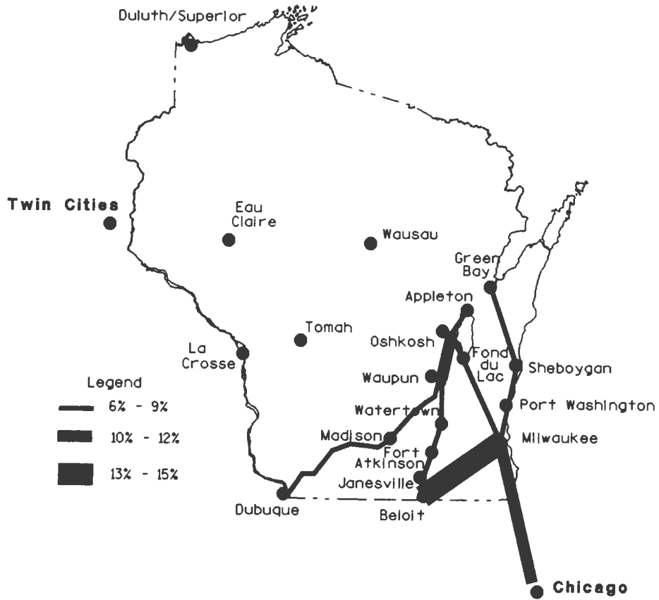
FIGURE 7 Impact of adopted plan on trend truck forecast, 2020: percent reduction in intercity truck volume.
