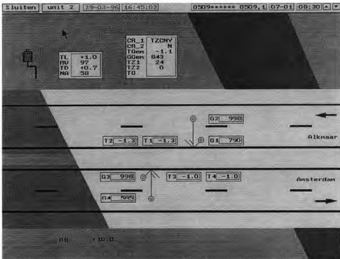
FIGURE 5 Illustration of measuring station, January 7, 1996, 8:30 a.m. Air temperature, humidity, dew point, and precipitation are shown in upper left box. Road temperature and conditions are shown at sensor locations in roadway. Note that road temperature is below freezing and air temperature is above freezing.
