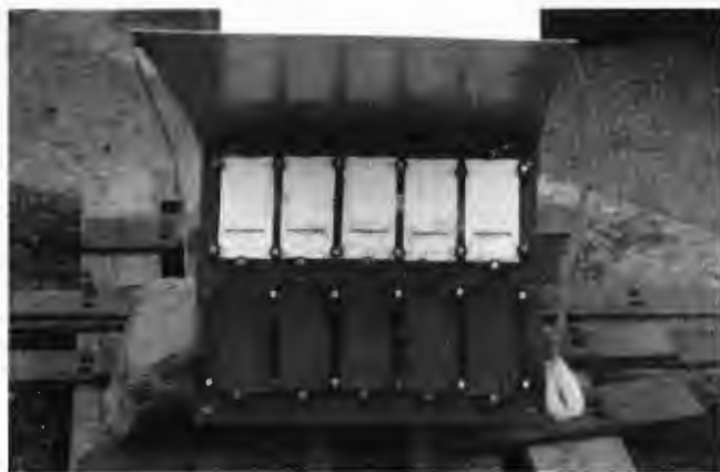
FIGURE 2 Steel plates, five painted and five unpainted, for corrosion test.
