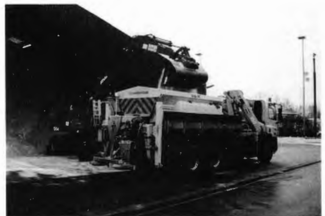
FIGURE 2 Truck with prewetting solution being loaded with salt in a maintenance yard.
