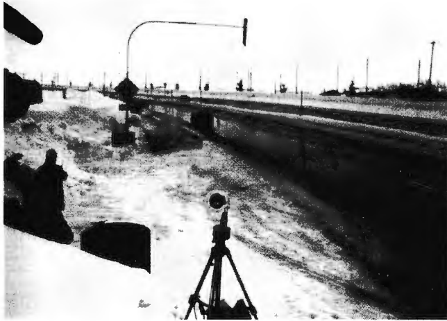
FIGURE 10 Field test of car halt surveillance radar on National Highway Route 12.
