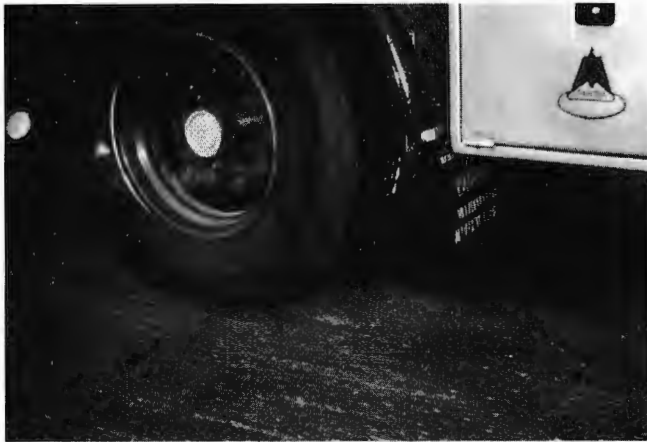
FIGURE 6 Air pumping effect of tires. Moisture visible behind tire has been sucked out of voids of porous asphalt. This effect transports thawing agent to surface and allows surface to remain wet.
