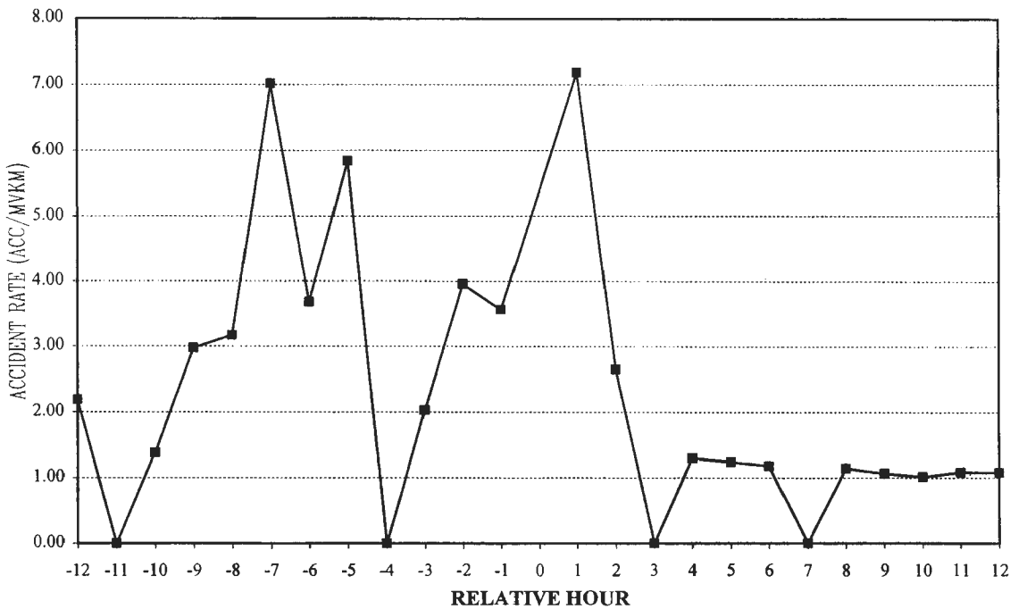
FIGURE 2 Accident rates for regular events, freeways.
