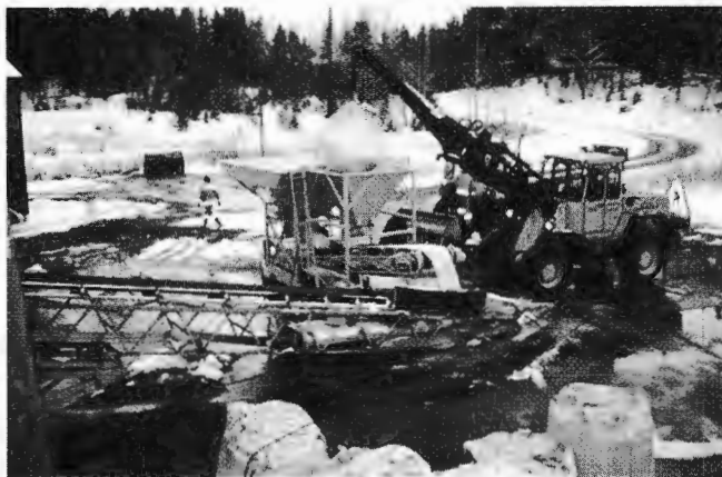
FIGURE 1 Mixing CMA-NaCl by using a small double hopper with conveyor belt.
