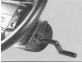
FIGURE 5 Relocation of transmission selector.
