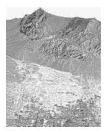
FIGURE 7 Fusion of ERS-2 satellite data (the background image) with ERS-1 data taken 3 years earlier (interferogram), both superimposed on TM 30-m data sharpened with SPOT 10-m panchromatic data. The interferogram shows an area of subsidence (at the millimeter level) near Las Vegas, Nevada, caused by groundwater withdrawal during the 3-year interval. (From *Professional Surveyor*, Oct. 1999.)
