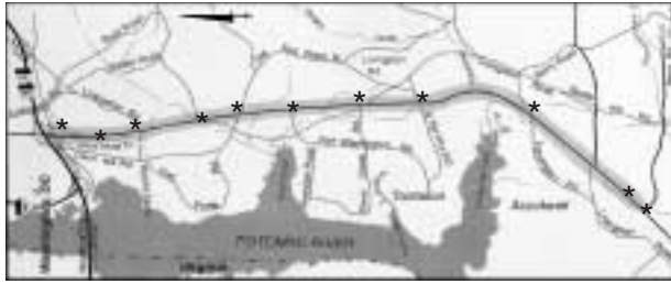
FIGURE 2 MD-210 corridor—overview: 10-mile corridor; 6-lane divided highway; 11 signalized intersections; clusters of suburban residential communities; commercial areas at existing intersections.
