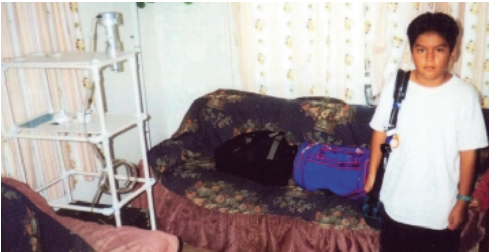
Figure 6. Child wearing personal monitor with separate sampler (left) for in-home monitoring of air toxics and fine particles.
