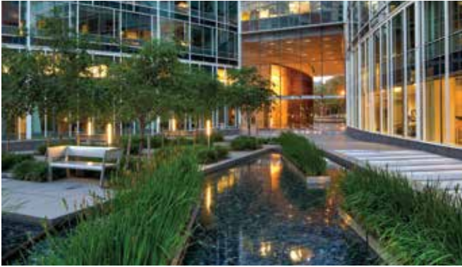
The attractive courtyard water feature holds captured runoff from the roof after it has been cleansed by the treatment system. (Sasaki)
