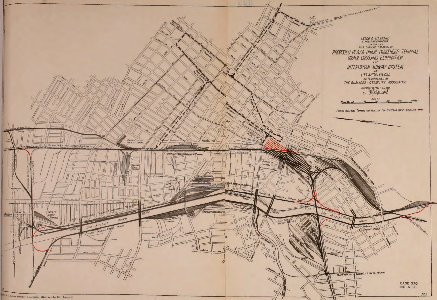
FIG. 114. BARNARD PLAN FOR UNION PASSENGER TERMINAL AT THE PLAZA This is the plan recommended by the Business Stability Association. This plan and the recommended Engineering Department plan makes use of the same site. Proposed immediate construction is shown in red.
