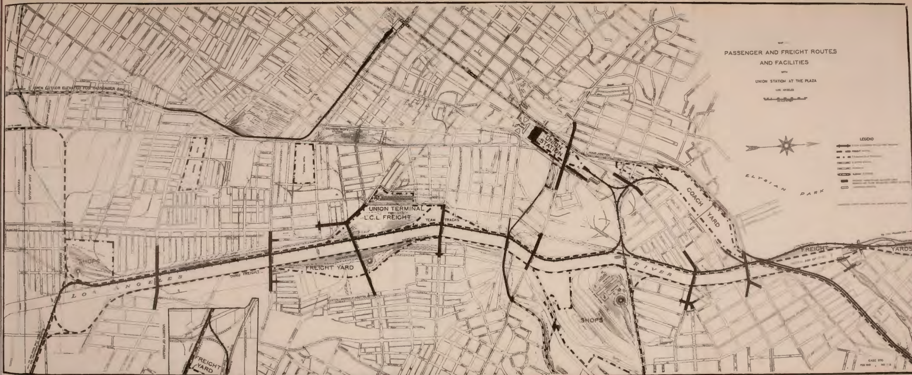
FIG. 180. NORTH MAP WITH UNION STATION AT THE PLAZA This plan has been made by the Engineering Department to show the location of passenger and freight yards and facilities as recommended. The passenger trains from the North and from Pasadena will head to the level of the freight yard and through. Trains from the East will reach the station directly along Alameda Avenue, and those from the south will run adjacent to the river on a new double track bridge. Through freight will use the east bank of the river.
