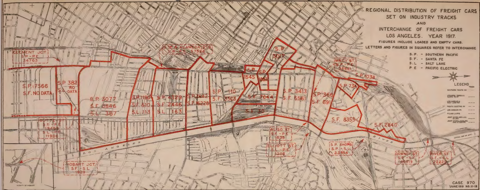
FIG. 107. REGIONAL DISTRIBUTION OF FREIGHT CARS SET ON INDUSTRY TRACKS, AND INTERCHANGE OF FREIGHT CARS LOS ANGELES, YEAR 1917. THE LOCATION AND SUMS OF TRAINS FOR EACH INTERCHANGE ARE SHOWN WITH THE NUMBER OF LOADED AND EMPTY CARS.
