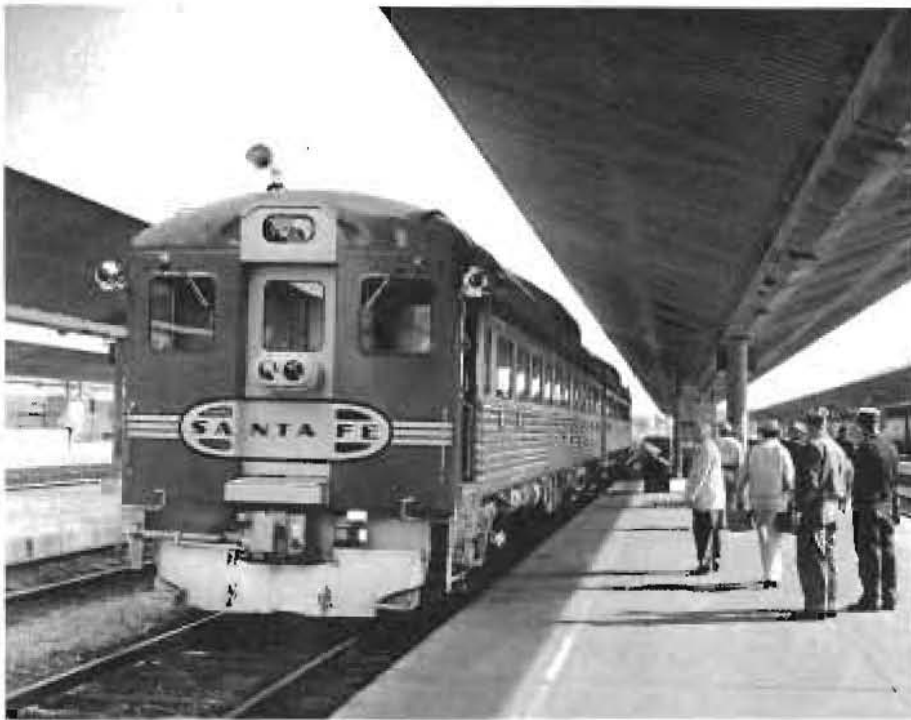
(Above) THIS PAIR of Budd RDC (Rail Diesel Car) self-propelled units served the Santa Fe's San Diego service during a portion of the 1950s.
