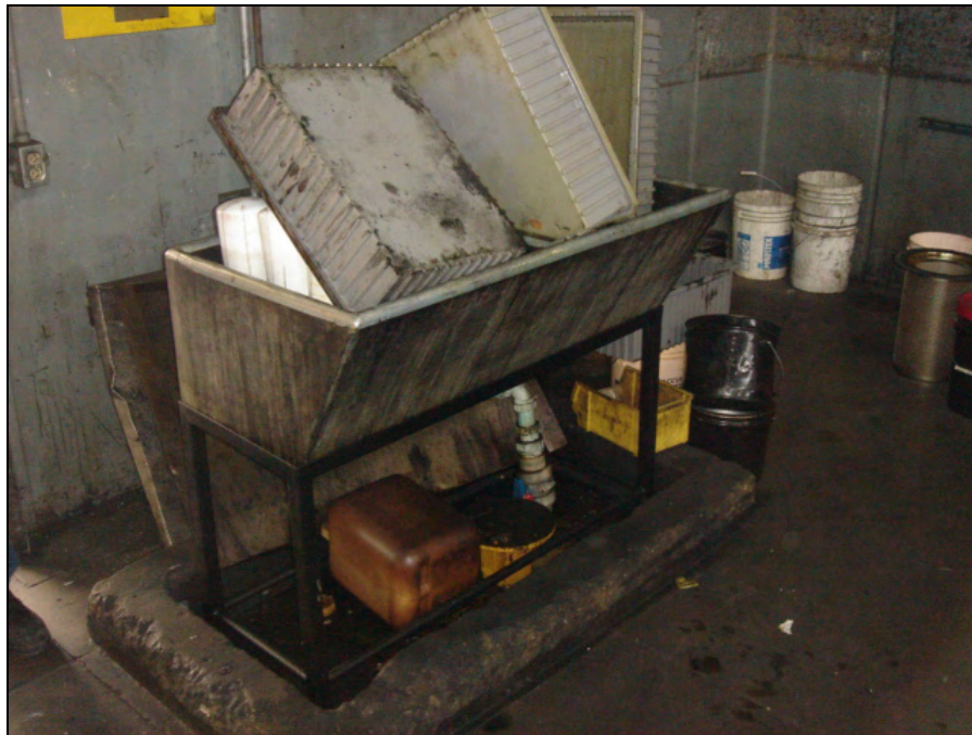
View of oil filter draining basin in Building 1
