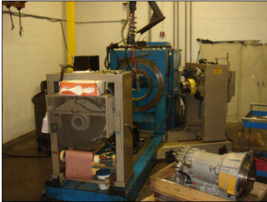
View of test station for rebuilt transmissions in Building 1
