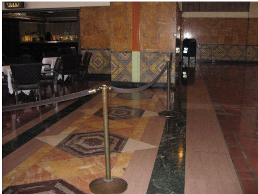
Barrier outlining the dinning tables with only one strap instead of two, as required.
