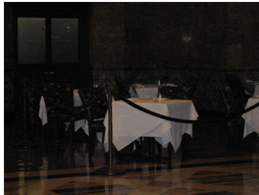
Barrier outlining the dinning tables with only one strap instead of two, as required.
