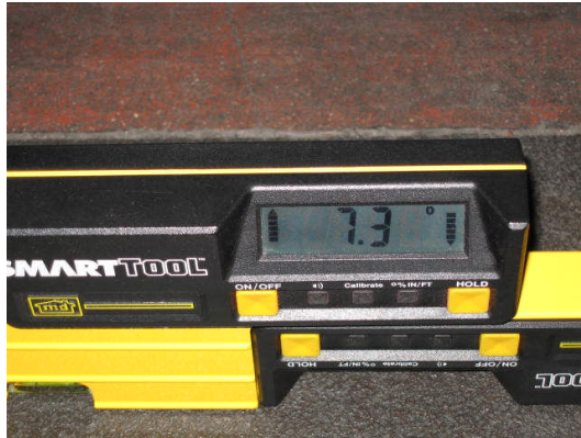
North ramps are within the 8.33% slope.
