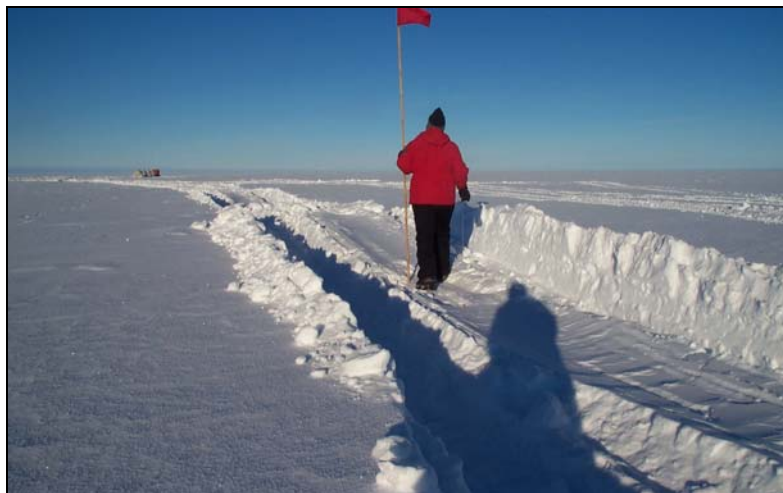
Figure 18. Deep ruts made after passage of four fuel sleds (full-empty-full-empty) towed in ruts of C95 over undisturbed snow. Dragging of tank saddle produced the sculpted center ridge, which can be higher than the undisturbed snow surface.
