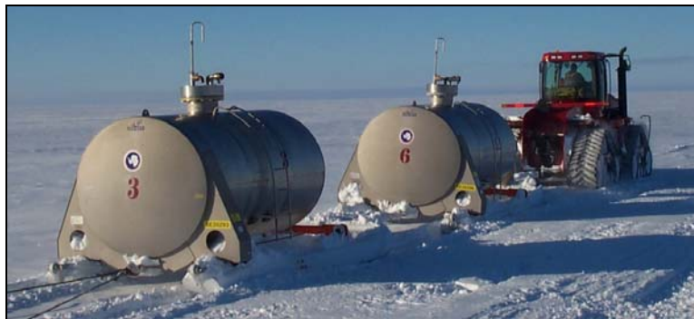
c. Two fuel sleds towed behind the Case tractor.
