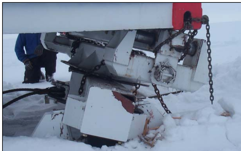
c. Holding bogies and containers together with chains.
