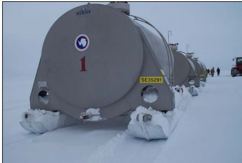
c. Case and C95 in Y-configuration pull tanks onto undisturbed snow.
