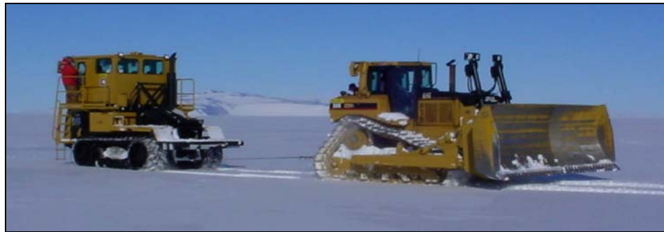
Figure 6. Dynamic drawbar measurement of Kress tractor conducted at 8 km/hr using D8R as load vehicle. Note that the Kress tractor towed through its drawbar (low hitch) not its fifth-wheel hitch.
