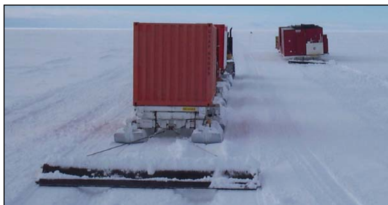
d. Dual-pipe and pipe-chain drags trailing sled trains.
