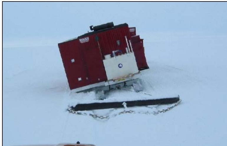
b. Roll of housing and energy modules.
