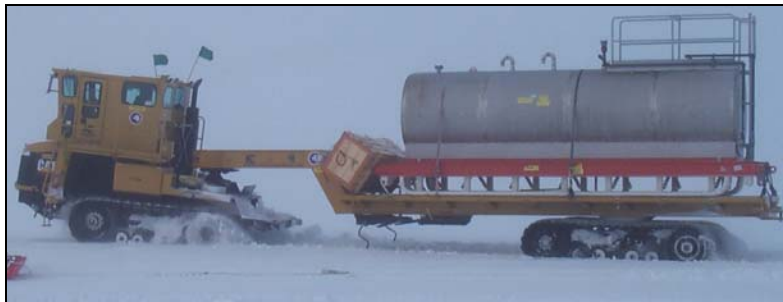
Figure 13. Kress tractor pulling tracked-trailer over undisturbed snow.
