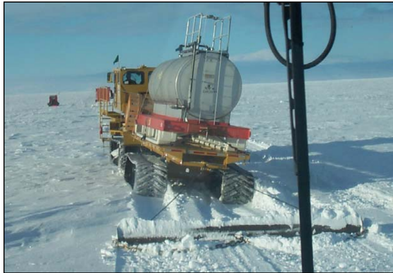
Figure 15. Large-amplitude roll motion of tracked trailer along trail northward.
