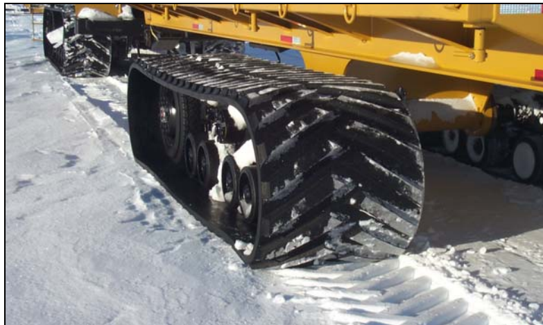
Figure 14. Tracked-trailer's insufficient lateral support of track by idler and bogie wheels.
