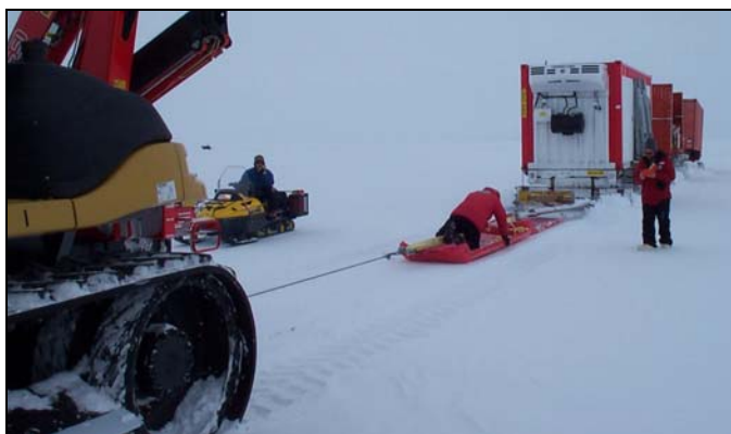
a. Three ISO sleds towed in the ruts of the C95 tractor.
