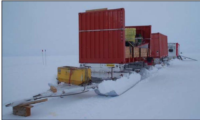
b. Three ISO sleds (flatbed, mil van, and refrigeration module).
