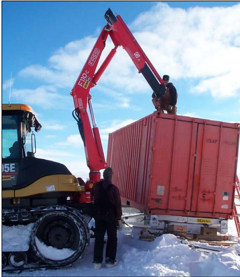
d. Placing container back on sled bogie.
