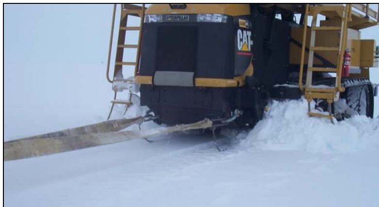
a. On undisturbed snow. Note the shallow rut left by the C95 when towing on undisturbed snow.
