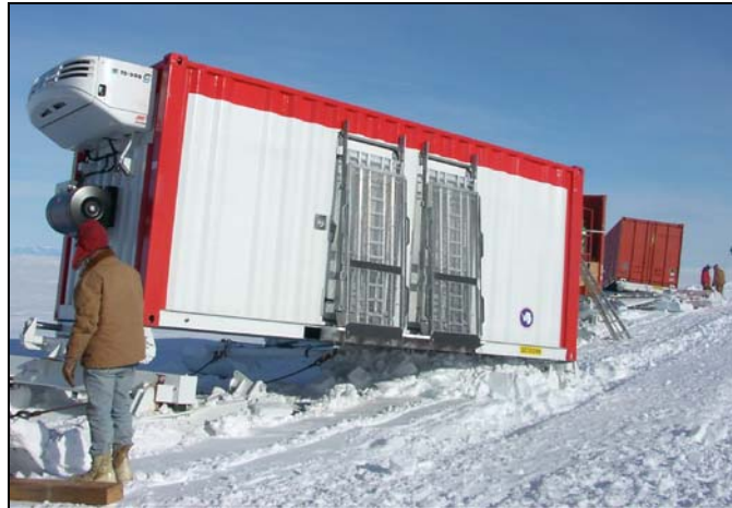
Figure 4. Large sled motions caused numerous failures of ISO sled attachment hardware, leading to “train wrecks.”
