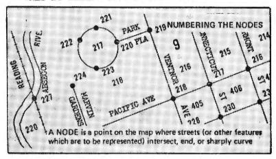
For each segment of a street (i.e., the length between two nodes) the GBF/DIME file contains the following information: the "from" node, the "to" node, the street type (e.g., avenue, drive, way, etc.) the address range on the right side of the street and the address range on the left side.
