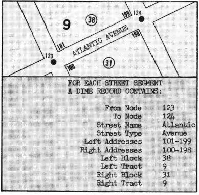
The term DIME, or Dual Independent Map Encoding, then refers to the fact that the basic file is created by coding two independent matrixes: a) the nodes at the end of the line segments and b) the areas enclosed by the nodes and line segments.
