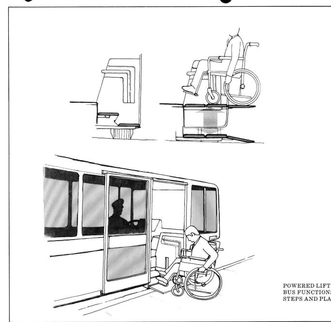
POWERED LIFT IN BUS FUNCTIONS AS STEPS AND PLATFORM
