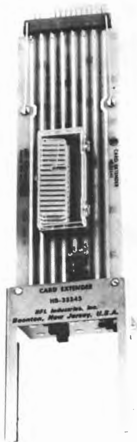
Figure B-5. Extender Board, P.C. View
