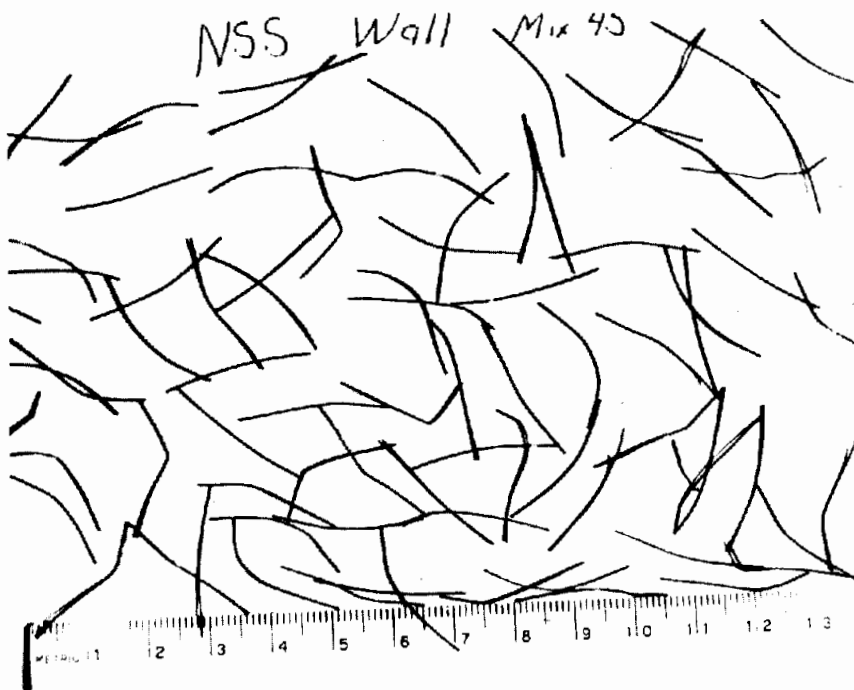
FIG. 3.7 TYPICAL NS FIBERS FROM FRESH SAMPLE OF IN-PLACE SHOTCRETE
