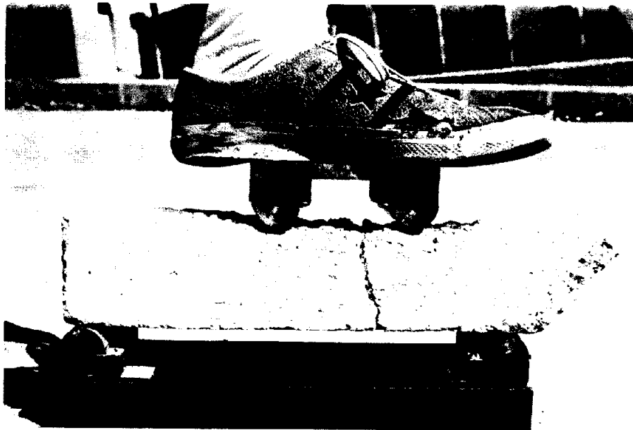
(b) Irregular open crack of a beam after testing
