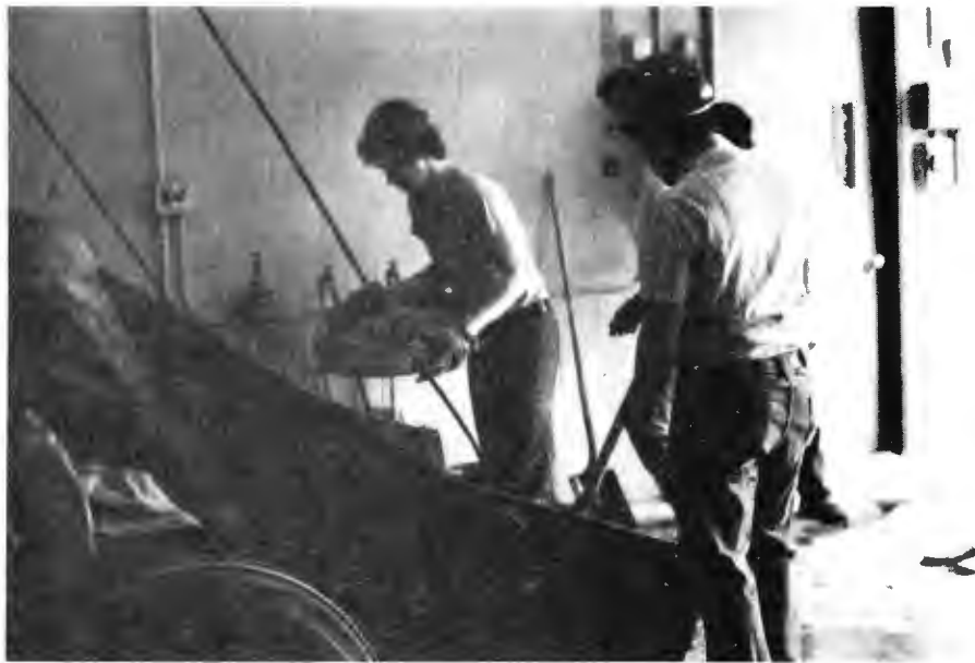
FIGURE 4.9 FIBER SCREENING USING 1-IN. (2.54 CM) SIZE SIEVE
