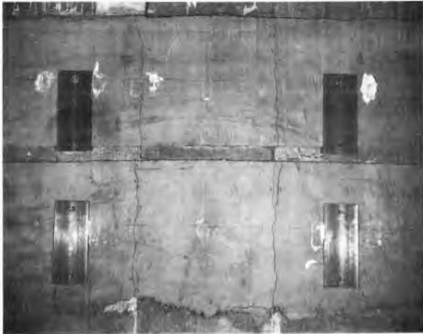
FIGURE 3.3 USE OF 6 X 18 IN. (152 X 457 MM) PLATES IN TEST NOS. 13 AND 14 TO SIMULATE ROCK BOLTING
