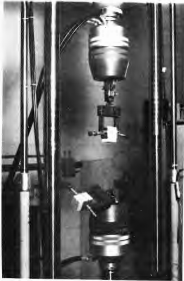
FIGURE C-3 FAILED ADHESIVE TEST SAMPLE
