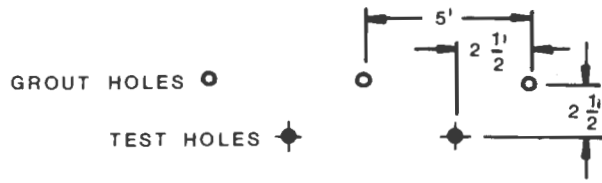
DETAIL OF GROUT AND TEST HOLES
