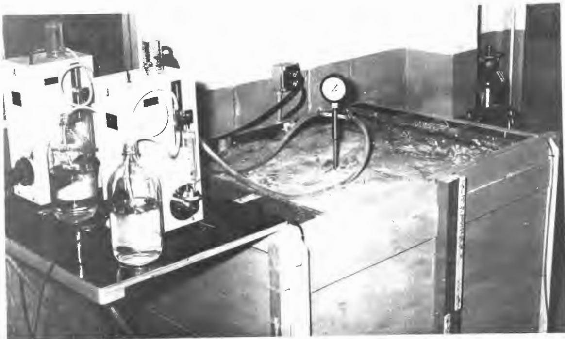
Figure D-4. Equipment for laboratory grout distribution test.
