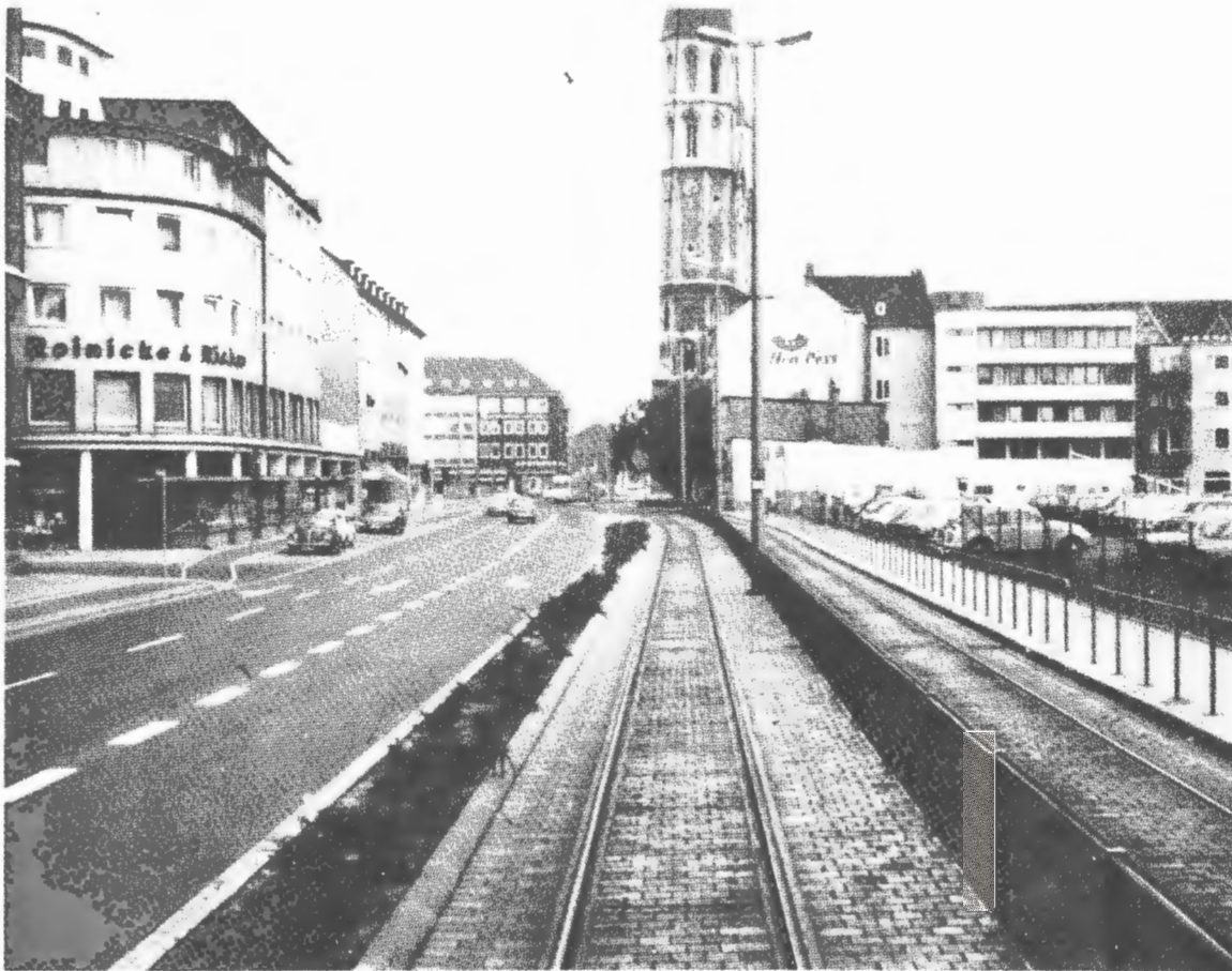
Figure 16. Separation of LRT Tracks and Traffic Lanes by Bushes in Brunswick
