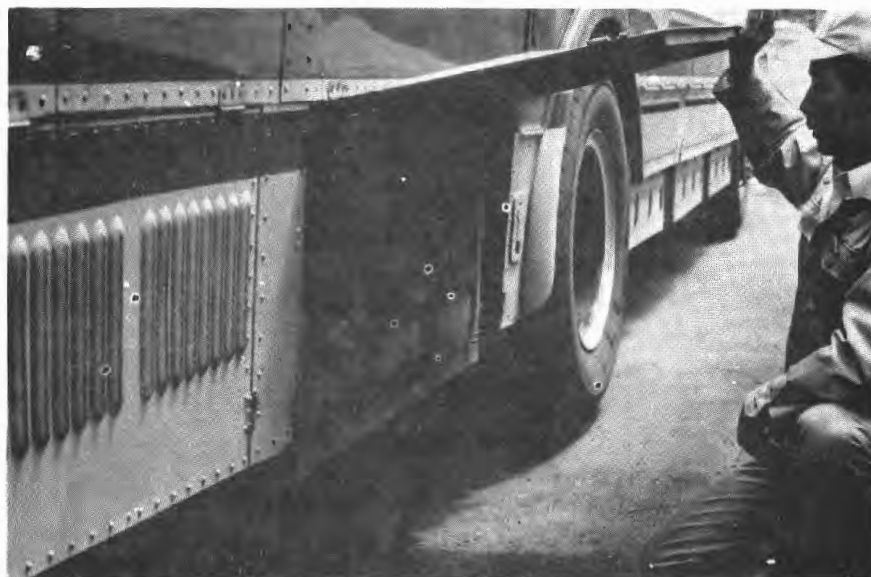
Figure 2-19. Battery Location, Mitsubishi Bus
