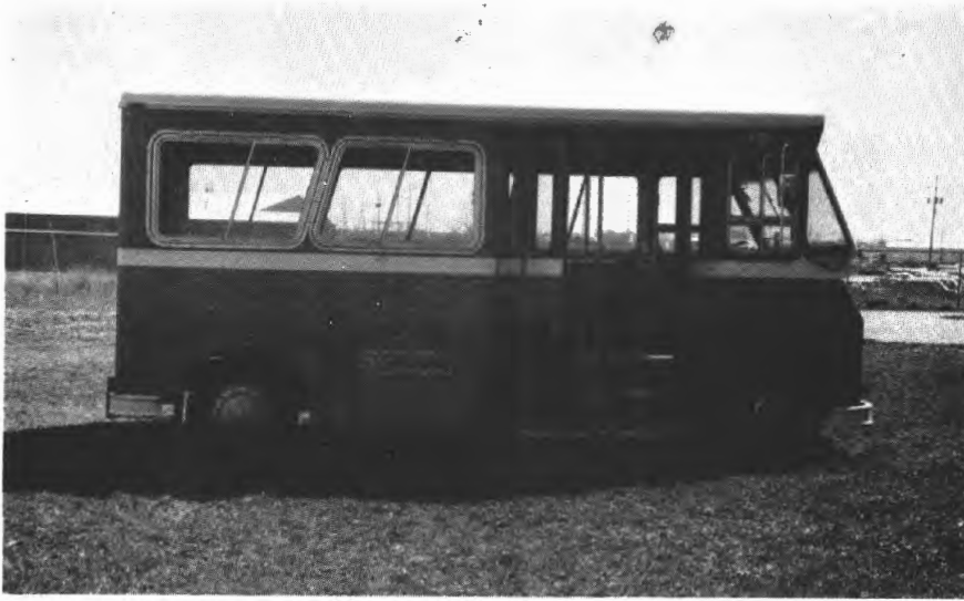
Figure 2-3. Battronic Bus, Showing 122-cm Wide Doors.
