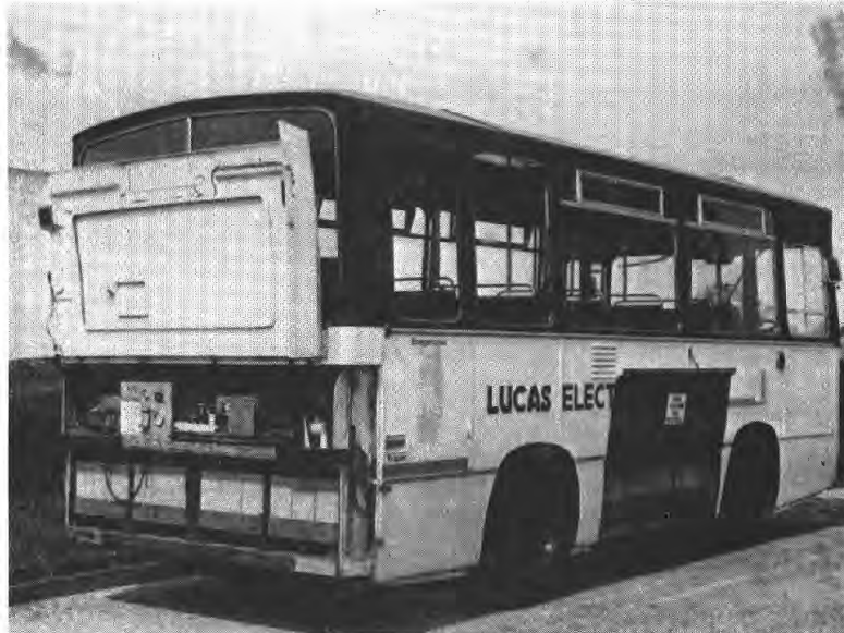
Figure 2-6. Rear View of Lucas Bus Showing Batteries and Controls
