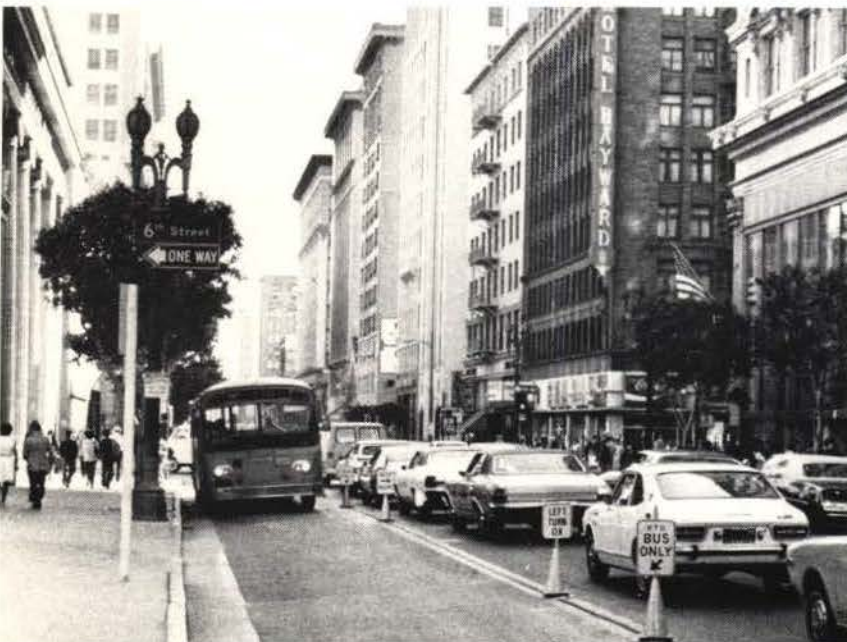
Contraflow Bus Lane, Los Angeles
