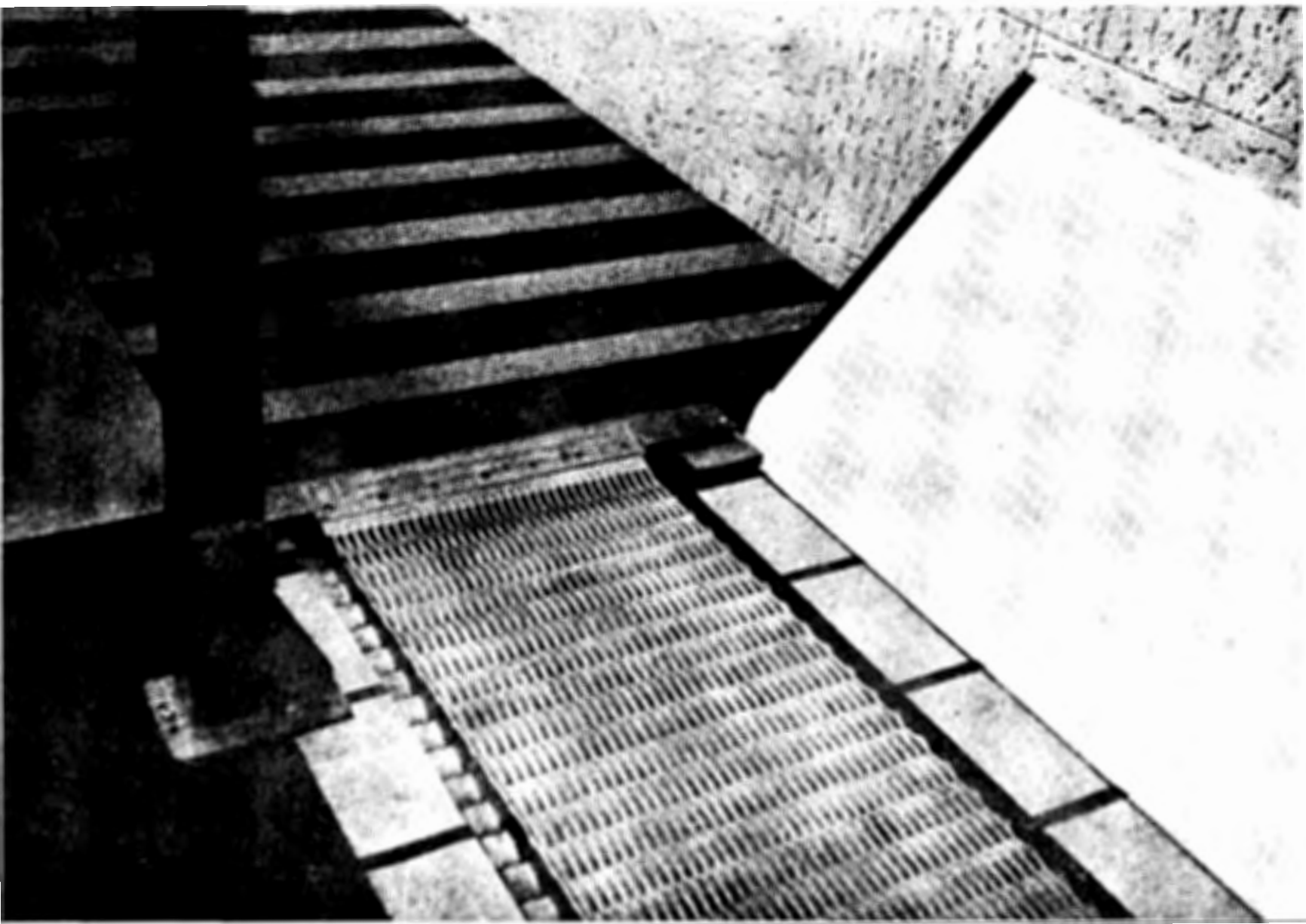
VIEW SHOWING STATIONARY COMBPLATE AT END OF PROTOTYPE UNIT.
