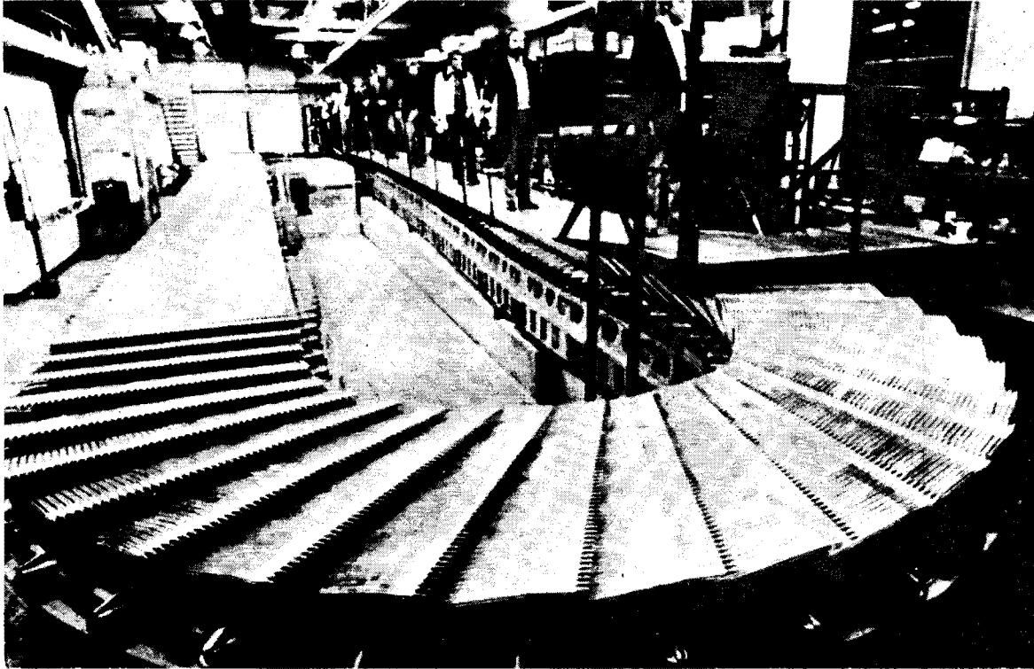
GENERAL VIEW OF TRAX PROTOTYPE LOOP. TREADWAY SURFACE FORMED OF GROOVED SLIDING PLATES, COMBING EACH OTHER AND COMBED BY STATIONARY COMB PLATES AT ENTRY AND EXITS.
