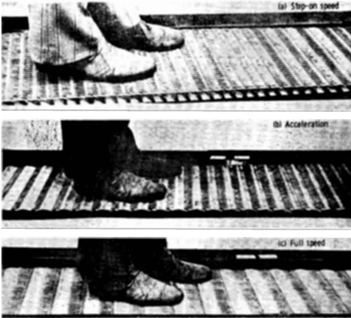
TREADWAY SURFACE. (a) STEP ON SPEED (b) ACCELERATION SECTION (c) CONSTANT HIGH SPEED SECTION.
