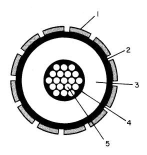
FIGURE 4. CROSS-SECTION, SAMPLE NO. A5-00-3 XL Polyethylene/Semi-Conductive Jacket/ 14 (3/16  $\times$  .027) tinned Cu armor over jacket. Outside diameter 25 mm.
