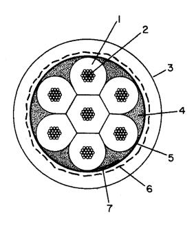
FIGURE 3. CROSS-SECTION, SAMPLE NO. A3-7X14-2 Proprietary compound/cloth tape, Neoprene jacket. Outside diameter 25 mm.
