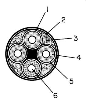
FIGURE 6. CROSS-SECTION, SAMPLE NO. A6-4X12-1 Silicone rubber-glass braid/Mylar tape/glass braid. Outside diameter 12 mm.
