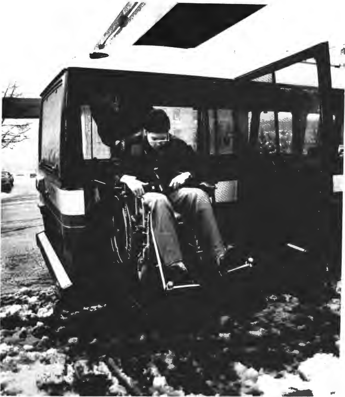
Wheelchair Lift in Operation, Portland, Oregon.
