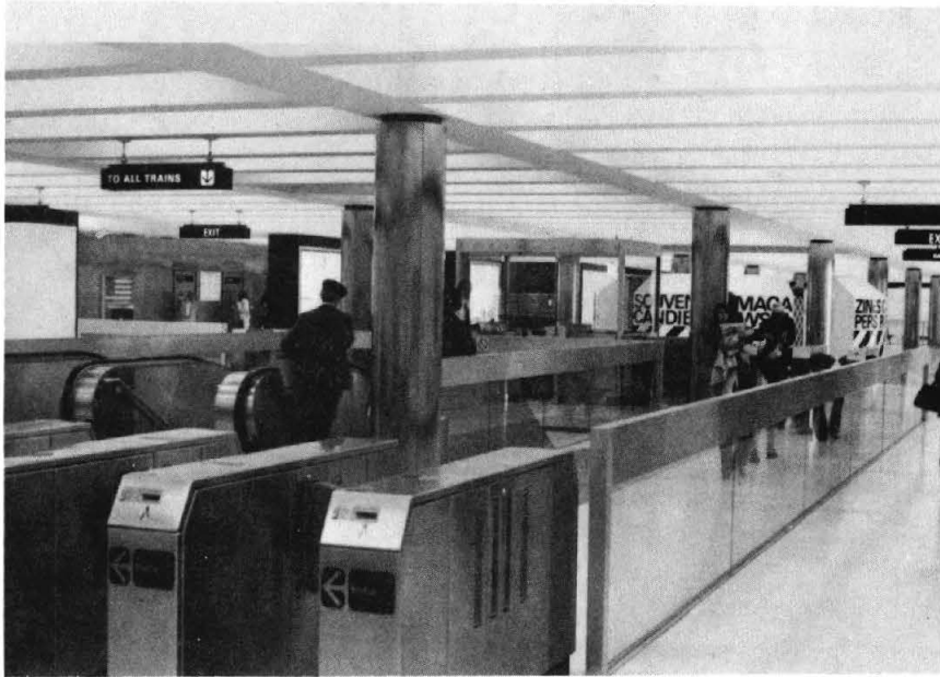
PLATE VI-6 LOW BARRIERS FACILITATING FARE EVASION, POWELL STREET STATION
