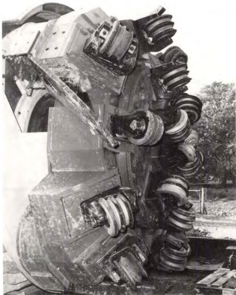
PLATE 2-6. Demag TBM equipped with triple discs
