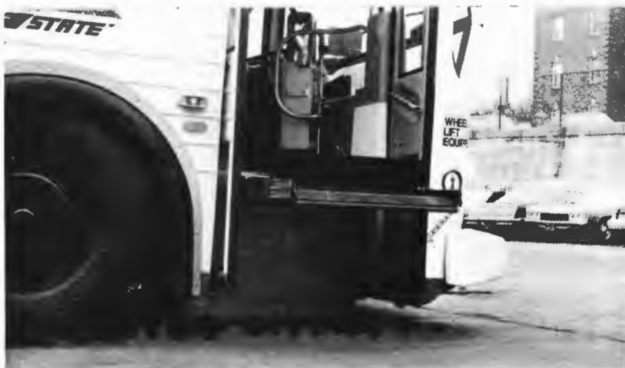
FIGURE 6-4 STAGES OF WHEELCHAIR LIFT DEPLOYMENT
