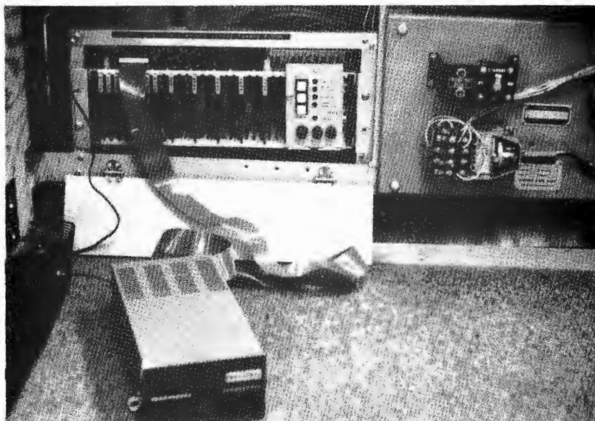
FIGURE 2.2.7. THE CONTENTS OF THE VEHICLE DATA ACQUISITION SYSTEM MEMORY ARE TRANSFERRED TO MINI-MAGNETIC DISK UNIT.
