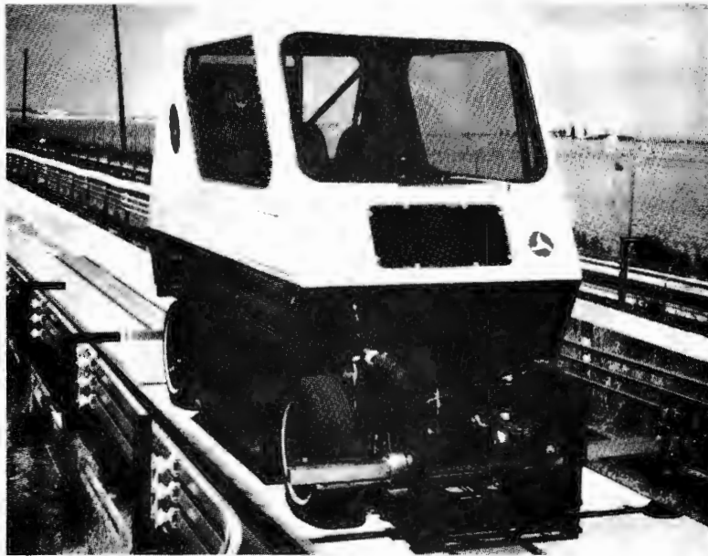
FIGURE 2.1.19. VARIABLE GEOMETRY LATERAL CONTROL SYSTEM TEST VEHICLE WITH A 2- OR 4-WHEEL DRIVE AND A SINGLE OR DUAL AXLE STEERING
