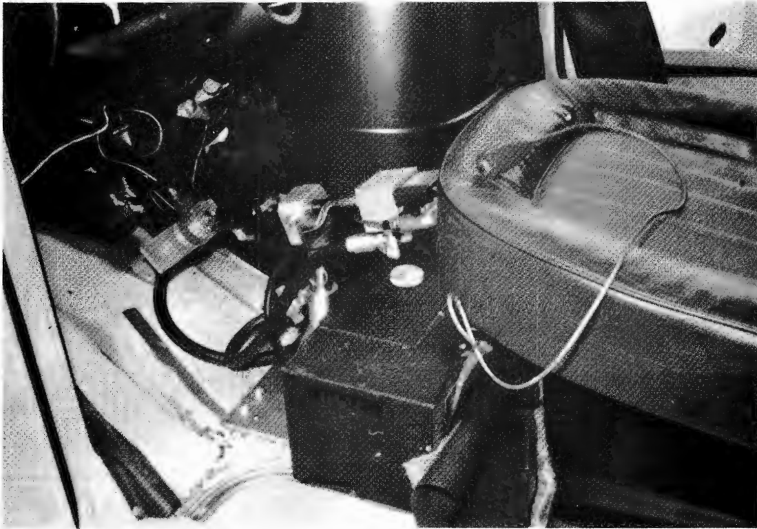
FIGURE 2.1.9. AN AUTOMATIC BRAKING CONTROL SYSTEM WAS USED IN THE DECELERATION TEST VEHICLE
