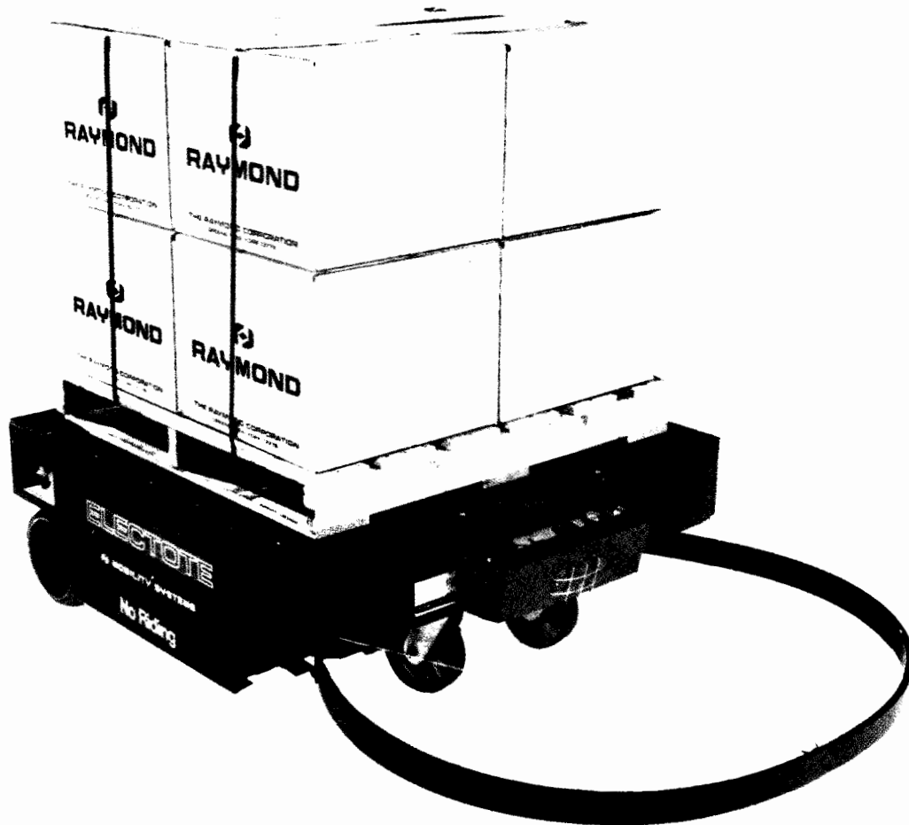
FIGURE B.1. SMALL INDUSTRIAL DRIVERLESS VEHICLE
