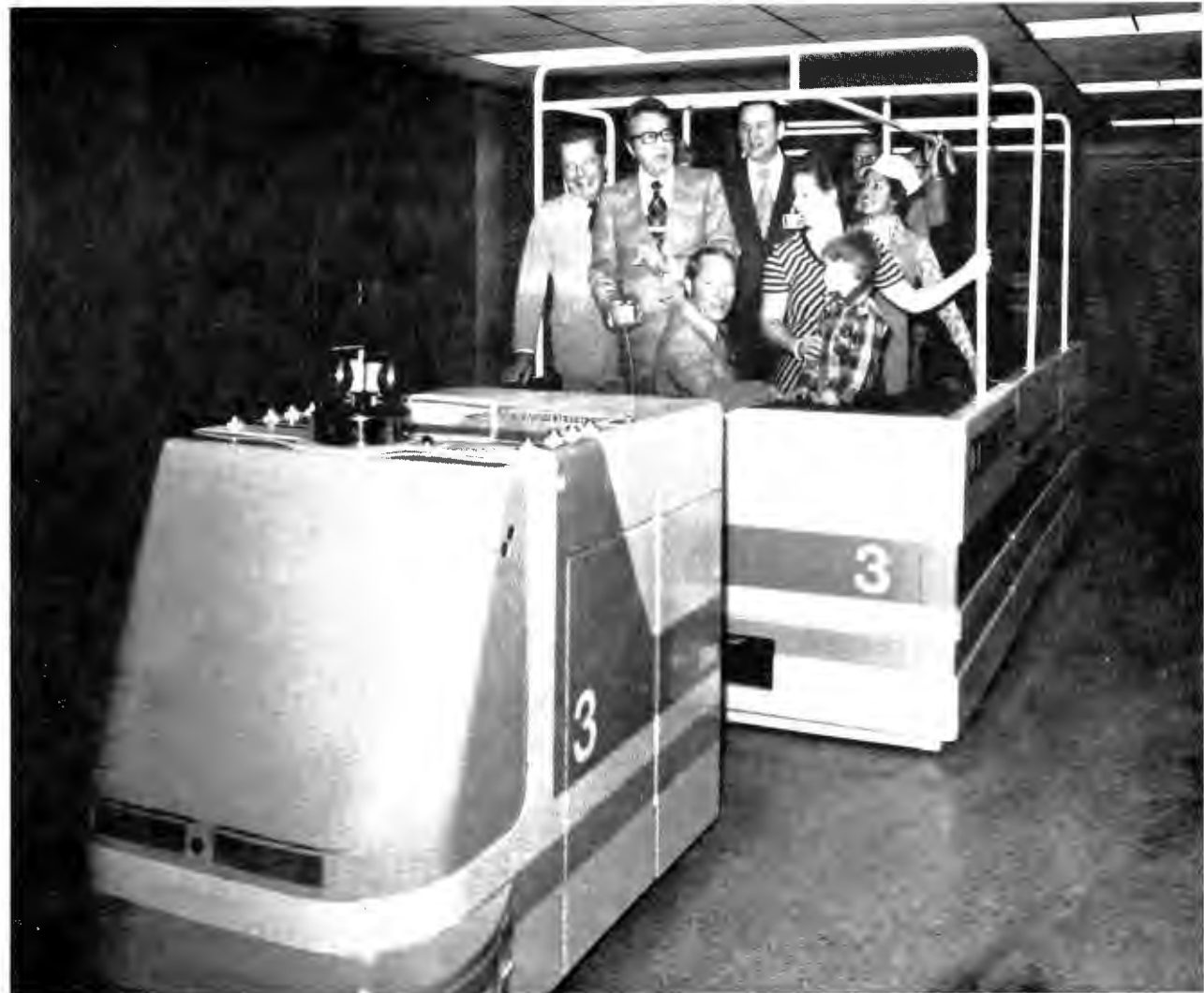
FIGURE A.3.2. FRONT VIEW OF OTIS AMTT VEHICLE
