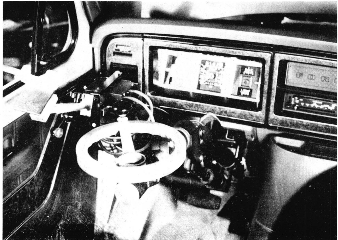
Equipment is now available that would enable 30 percent of all wheelchair users to drive cars. The photographs show the control mechanisms for two lift-equipped vans that can be operated from a wheelchair. Left: hand-controlled lateral steering, acceleration, and braking require one-twentieth the effort of standard controls. Right: knee-controlled lateral acceleration and braking (showing electric wheelchair control at lower right.)
