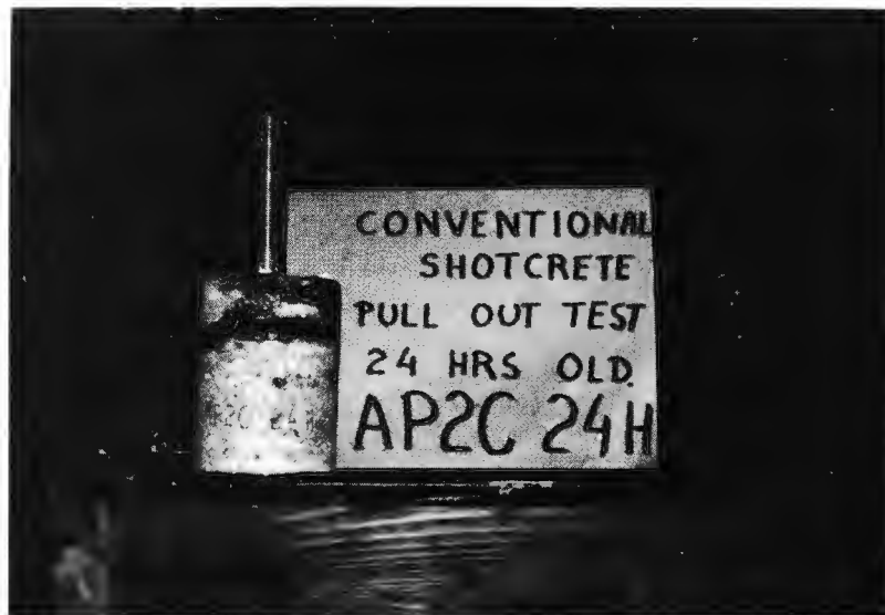
Figure VIII-18: Pull-Out Cylinder of Shotcrete.
