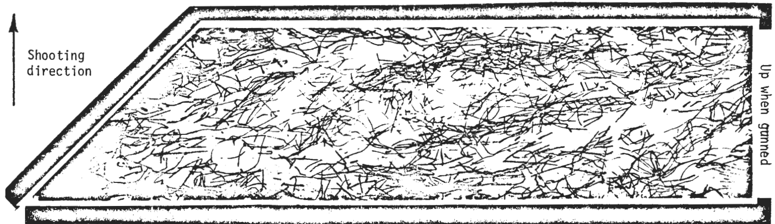
TYPICAL X-RAY PHOTOGRAPH OF STEEL-FIBER-REINFORCED SHOTCRETE
