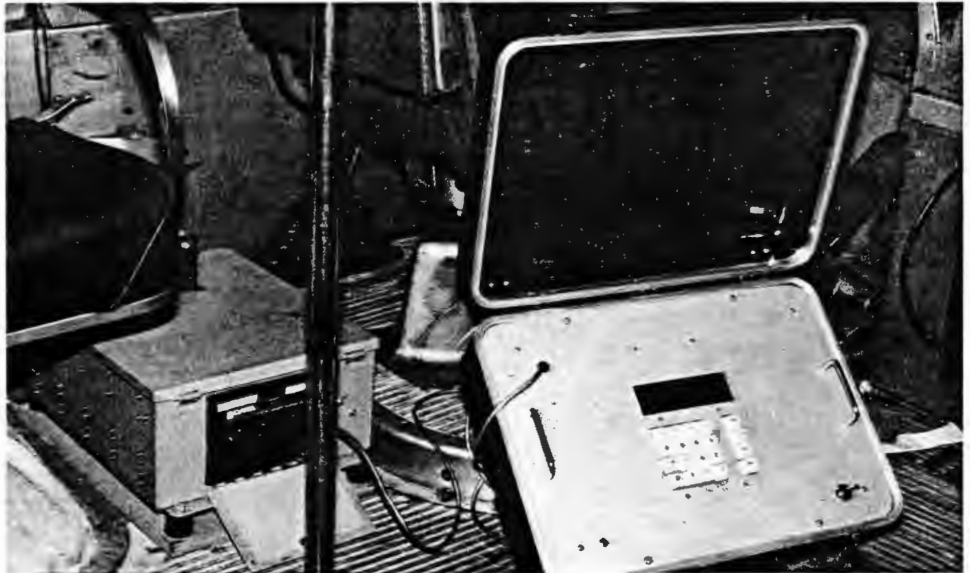
The portable data collection unit demonstrated in Columbus provides information on passenger loads, run times, and schedule adherence. (Photo by General Motors)
