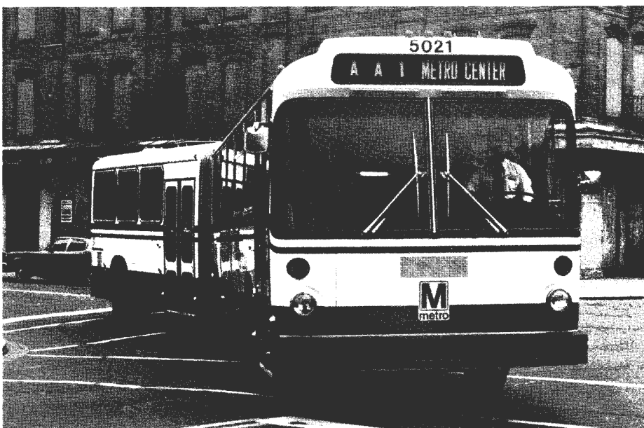
Articulated buses with bending characteristics can carry more passengers down congested streets
