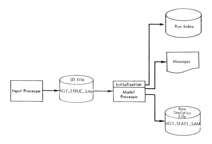
FIGURE 2-2. MODEL PROCESSOR - DATA BASE INTERFACE
