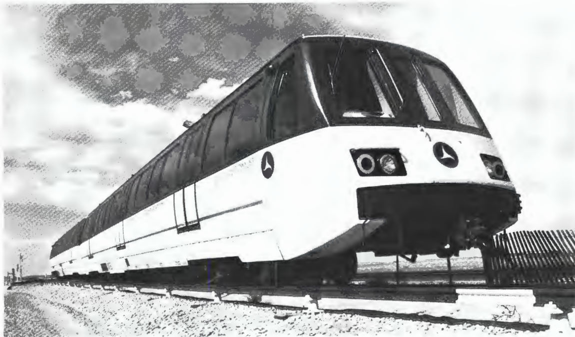
This experimental vehicle, the Advanced Concept Train (ACT-1), was developed for UMTA to evaluate advanced transit car systems for improved safety, performance, and operating economy.
