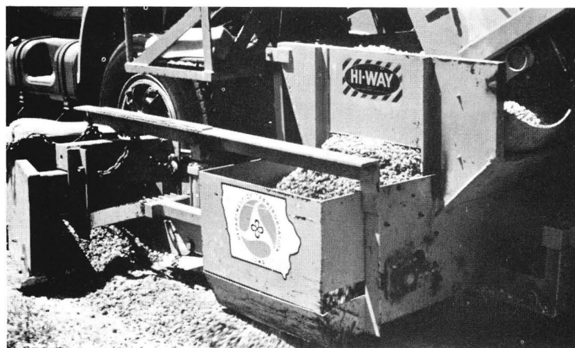
Side Delivery Shoulder Spreader Developed by Iowa DOT
