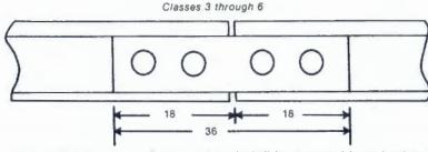
Each rail joint in Classes 3 through 6 track shall be supported by at least one crosstie specified in paragraph (c) of this section whose centerline is within the 36" shown above.
