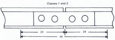
Each rail joint in Classes 1 and 2 track shall be supported by at least one crosstie specified in paragraph (c) of this section whose centerline is within the 48" shown above.
