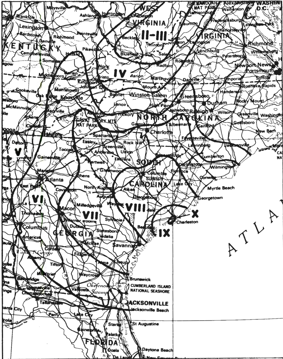
Figure 10. Isoseismal M.M. contours for the Charleston, 1880 earthquake. (After Bollinger)
