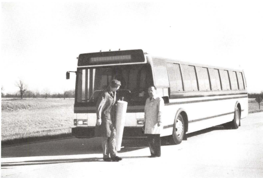
FIGURE 4.5. GRAVIMETRIC TANK AND GRUMMAN CONTROL BUS
