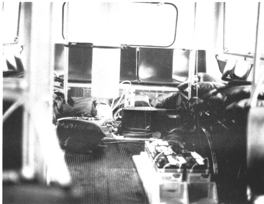
FIGURE 4.10. TEST FUEL SYSTEM INSTALLED IN BUS
