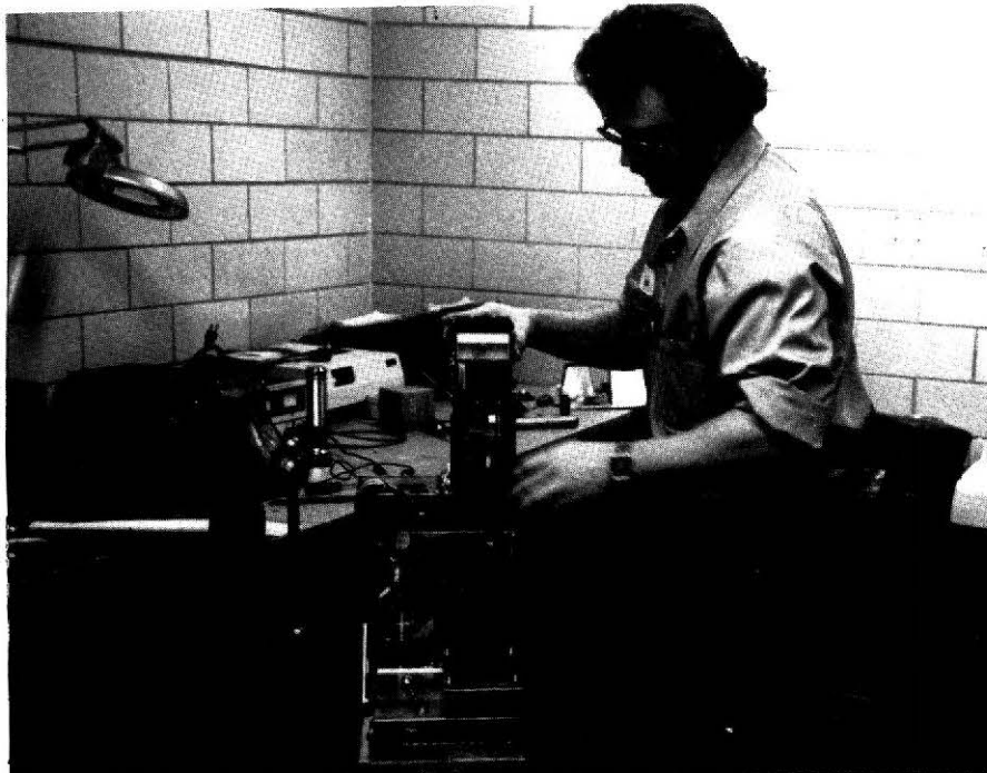
FIGURE 6-1. BILL TRANSPORT BEING REMOVED FOR PREVENTIVE MAINTENANCE AT DALLAS TRANSIT SYSTEM
