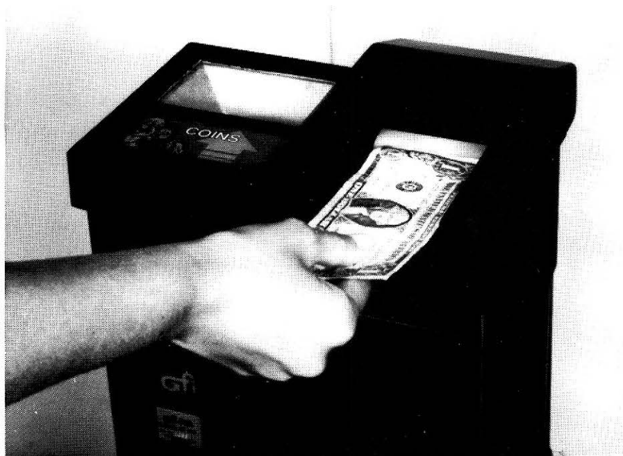
FIGURE 2-6. BILL ACCEPTOR ON GFI FAREBOX
