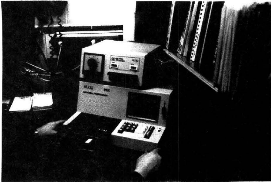
FIGURE 3-7. UNIVERSAL PROM PROGRAMMER AT MSBA
