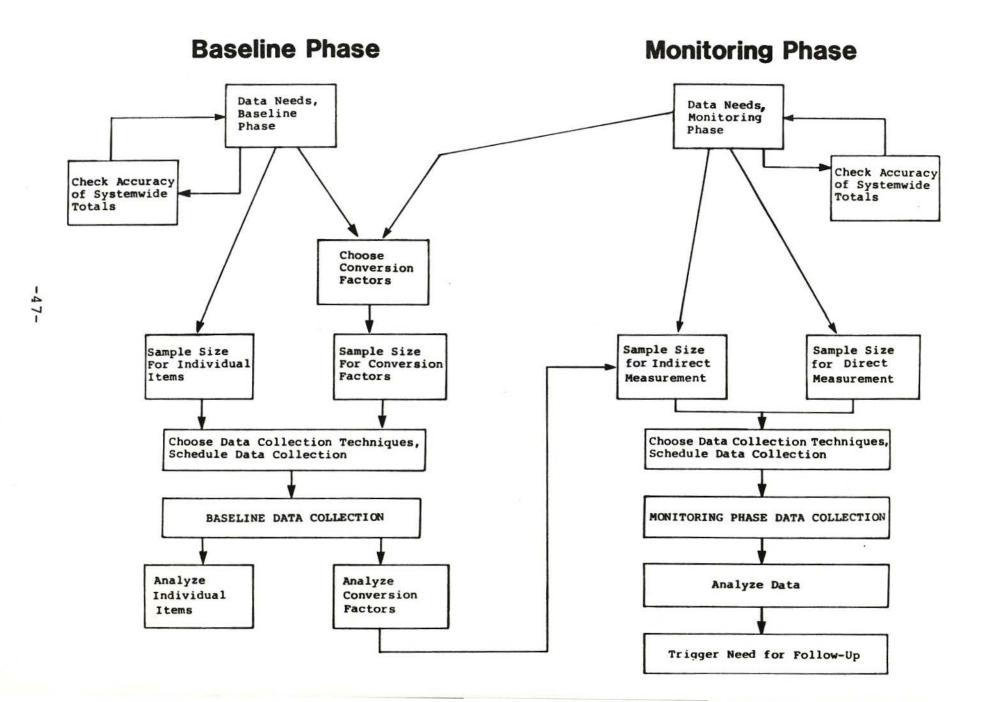
The first step is to define data needs for both phases, as described in Chapter 2 and in Sections 4.2 and 4.3. Part of the definition of data needs is the specification of accuracy level, a topic covered in Section 5.1.1. The chosen accuracy level for route-level items must then be tested to ensure that, when the data are aggregated to yield systemwide totals, the systemwide totals will be accurate enough. This topic is covered in Section 5.1.2.
