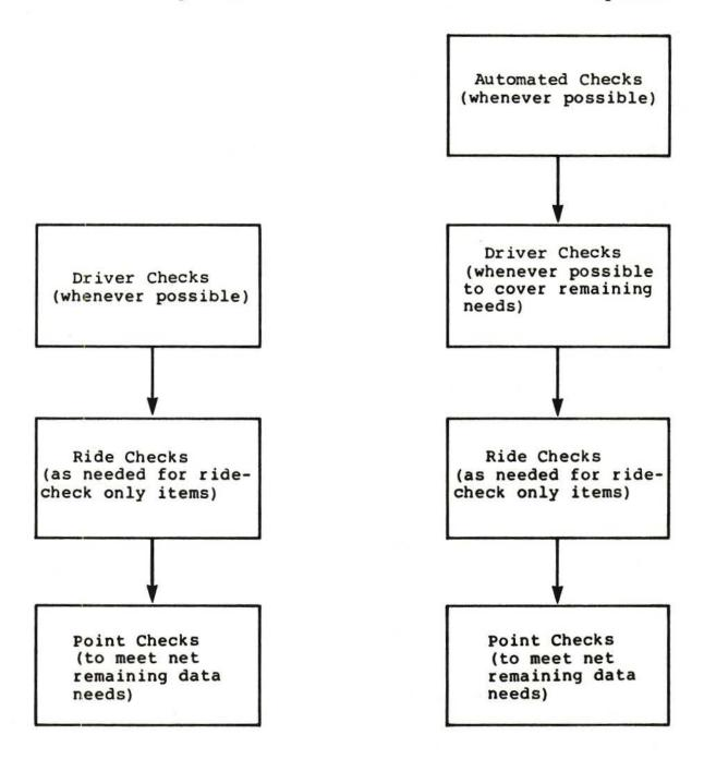
samples obtained via ride checks). For example, if boardings, measured using ride checks, requires a sample size of 9 trips while load at the peak point requires 20 trips, 9 ride checks are scheduled, and are supplemented by 11 point checks at the peak point.
