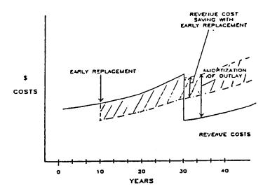
The effective cost saving from early replacement is thus the shaded area. Although the shape of the curve after the originally scheduled replacement in year 30 is rather indeterminate for present value calculation purposes (allowing for heavily discounted effects in later years), it is again reasonable to make initial annual savings x expected life of replacement asset as a first approximation.
